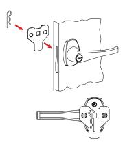
With the handle still in the open position, hook the locking bars (Ref. No. 12) to the locking cam (see "A" at left). Once in position, slowly rotate the door handle to the closed position so the lock bars prot rude from the holes at the top and bottom of the door (shown at right, below).
