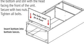
9. Using two people, set the unit upright and insert the partition (Ref. No. 10) into the cabinet, alining the four holes in the partition with the holes in the cabinet bottom and the cabinet shelf. Attach with four bolts and nuts, making sure that the bolts are inserted from the top downward to prevent stored items from being snagged.
