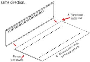
**4.** Attach the right side (Ref. No. 3) to the back in the same manner as you did in step 3, again, making sure that the flange is around the back and that the lances on the shelf adjustment strips are pointed in the same direction as those on the back and left side.
