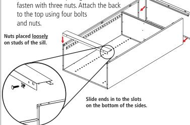
7. Next, attach the sill (Ref. No. 6) to the sides, as shown above. Place nuts loosely on each of the studs and slide the ends of the sill into the slots on both sides of the unit. Then, securely tighten the nuts.
